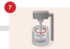
7 結晶と蜜を振り分け Spin the crystals in a centrifuge to remove liquid
